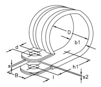
$\begin{array}{lll} \text{b1} & = 31.0 \\ \text{d} & = 10.5 \\ \text{Diameter D} = 70 \\ \text{h1} & = 52.5 \\ \text{I} & = 10.0 \\ \text{s} & = 1.00 \\ \text{s2} & = 3.0 \\ \text{Width B} & = 25 \\ \end{array}$
